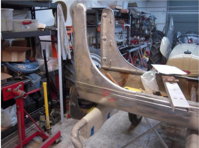
The rear section of the hood needed to be completely replaced as it was oriented in a cocked manner that prevented it from mounting without a large gap on one side. I used a flat plate of 1/8" 5000 Aluminum sheet that I cut and drilled to match the dash.
