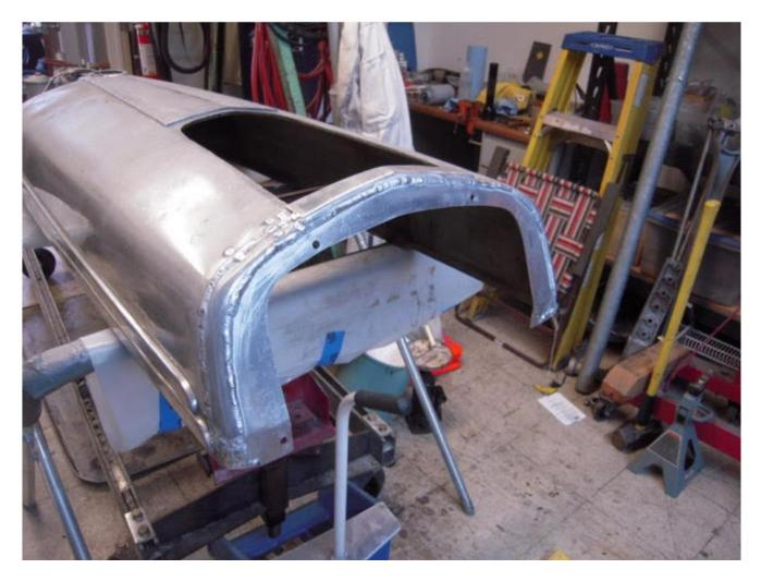
First fitting after grinding and sanding the welds, everything lined up pretty well, and the attachment tabs on the dog legs ended up where they should although some material needs to be added for the lower attachment hole to be drilled properly. The upper hole works fine.
