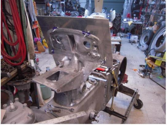
The result of the welding. I had to take a slim section out of the left side of the hood to make it properly square as can be seen in this photo. That was a real scary part, and I cannot explain why it was necessary, but it was.
